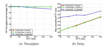
Fig. 6. Performance of the eBDP algorithm as the RTT of wired backhaul is varied. Data is shown for 1, 10 downloads and 0, 10 uploads. Here the AP throughput percentage is the ratio between the throughput achieved using the eBDP algorithm and that by a fixed buffer size of 400 packets (i.e. the maximum achievable throughput in this case).
